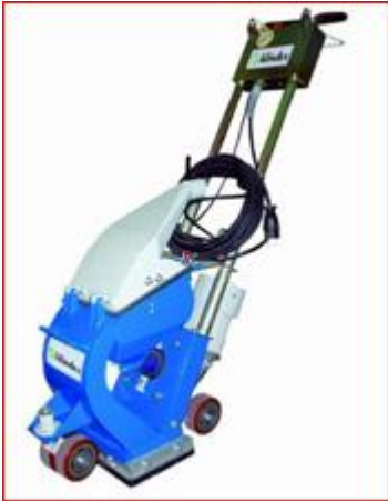
A Typical Small Vacuum Blastcleaning Machine and Dust Extraction Attachment for Concrete Floor Preparation
