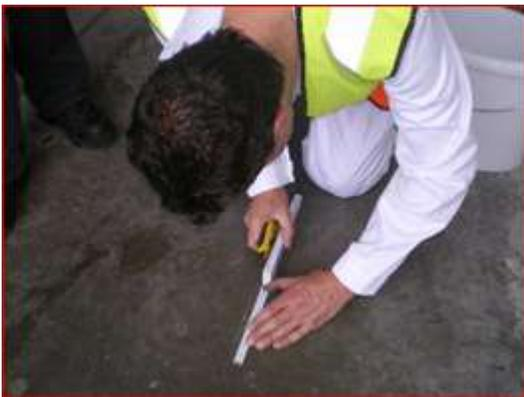
Surface Scratch Test – No visible / significant cut dimensions
